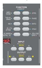
and make the measurement. Selection of analog and digital inputs is clearly indicated on the front panel with LED legends. Portable One makes graphs of swept measurements in real time
